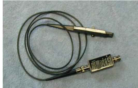
Figure 34 — Scope probe used for current pickup.
