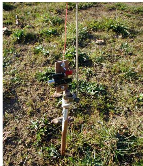
Figure 29 — Feed point and ground rod of test antenna #3.
