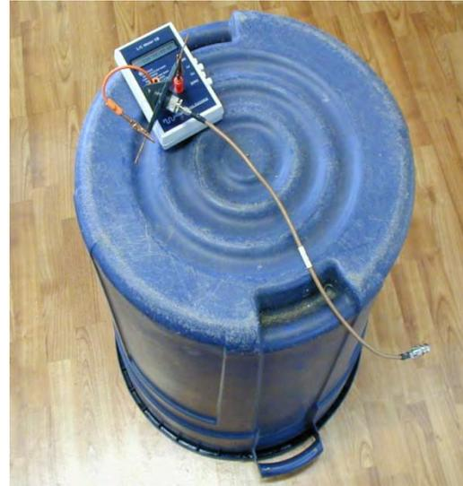
Figure 3 — Shunt capacitance measurement of the center fitting.
