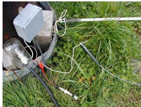
Figure 35 — Base excitation and current sampling example.
